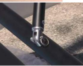
Locate the tiller extension and secure it to the tiller crossbar using the clevis pin and ring clip provided.
