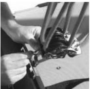
1 Connect the main sheet block to the traveler car. Attach the shackle that is part of the block through the clevis pin on the traveler car. Hook the mainsheet to the clew grommet at the rear of the main sail.
