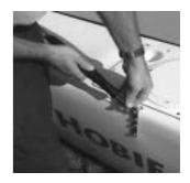
Attach the furler to the two bridle wires. Make sure the hole in the furler housing points towards the front crossbar. Wind some line onto the furler drum - 10 turns or so.
