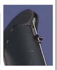
As shown, shackle the halyard to the top of the sail. Feed the top portion of sail into the mast track opening. Begin pulling on the halyard line. Use caution to be sure the sail feeds smoothly into the mast while raising. When the sail is all the way up, position the stopper on the wire halyard so that it engages in the halyard lock. Attach the main halyard rope to one of the white cleat at the bottom of the mast.
