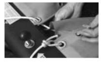
Tie a bowline knot to the forward left/port grommet in the trampoline. Pass the line through the opposite grommet, top/down and then through the lacing flap. Come up through the next (left) grommet and then continue to lace towards the aft of the trampoline following this pattern (down through the right grommets and up through the left grommets). Keep the laces loose at this time. Lace as far aft as the line will go.
