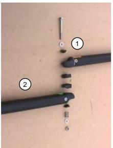
Locate the tiller crossbar and identify the left and right hand ends. NB: the tiller crossbar (1) locates on top of the tiller/rudder arms (2).
