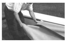
Slide the main trampoline bolt ropes into the hull trampoline tracks. Soapy water can be used as a lubricant (Do not use an oil or silicon lubricant on the trampoline track or the bolt rope). Sliding the bolt rope into the track is a 2 person job. One person should pull the trampoline and the other feed the bolt rope into the track.
