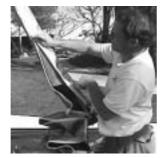
The jib is furled on the forestay and covered by a snorkel. To remove the snorkel, simply unzip as it is pulled down.
