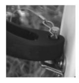
Insert the retainer pins to lock the rudders in place. The pins will prevent the rudders from falling off the boat in the event of a capsize.
