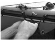
Pull the lace lines under the cross bar and tight. Begin the aft lacing by routing the left line up and over the first lace peg. Cross over to the next peg then down and around the rod. Pull the lace line tight then up and over the peg and then over to the next one and so on... Then start with the right side and work towards the center. When you reach the center, the pattern must be changed
